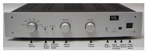
You can operate the various controls and switches from the front panel to access the full functionality of the unit. The Status indication LED shows the various operating modes of the unit.
